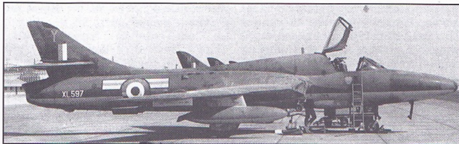
One of 208's Hunter T7s (two others during the Squadron's tenure in the Middle East were XL565 and XL602), standing on the apron at Khormaksar, in Aden. The observant will note that the outer stores pylons are fitted with jettison guns (the small blister on the upper surface of the wing gives it away), which was not a common modification on T7s.
