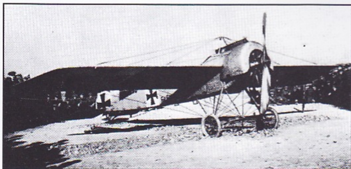
This aircraft is a Fokker "Eindekker", the Germans' best fighting machine in the first year-and-a-half of the War, as it had a synchronised gun. This one is in fact an E.III, with a Spandau gun and 100hp engine.
