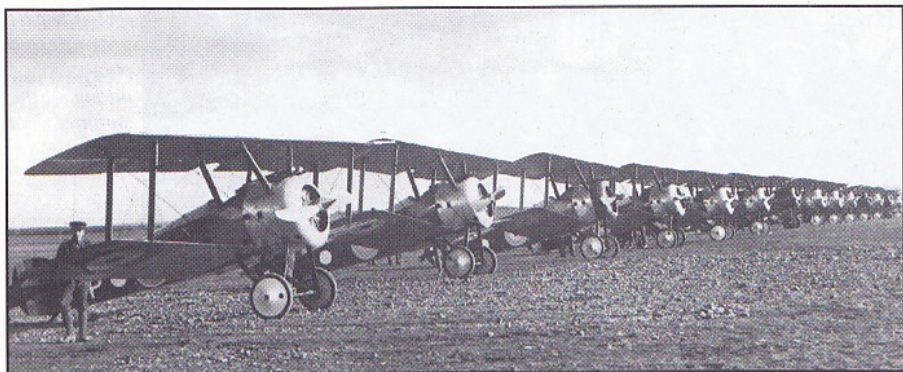
Shortly after relocating to Mont St Eloi, Naval Eight exchanged their trusty Triplanes for Sopwith Camels. Fourteen of the new aircraft are seen here. These would have been Clerget 130hp engined examples, most built by Sopwith, but some were from Clayton & Shuttleworth production.
