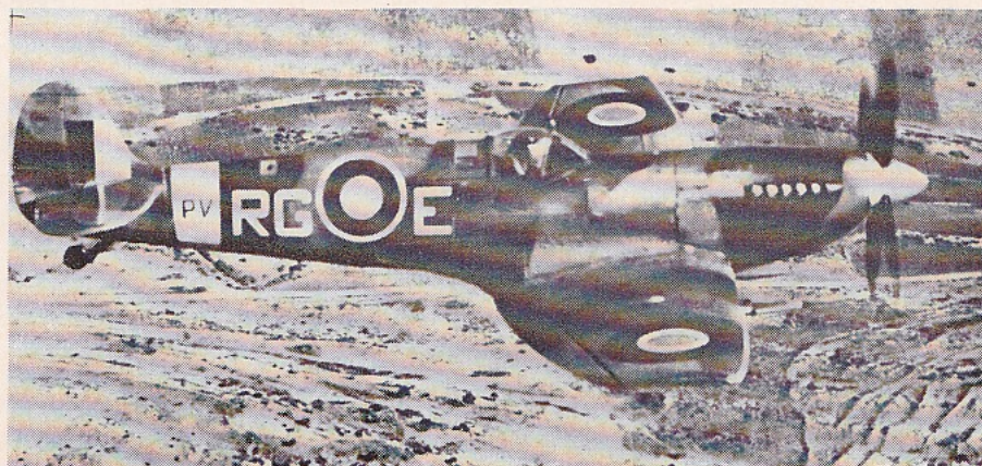
No. 208's mount during the Italian campaign, and for the rest of the war, was the Spitfire IX. PV117 illustrated is a clipped-wing LF.IXE
